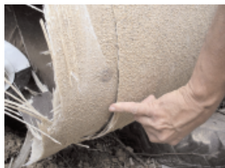
Upgrading Old Pipelines in Zone 3 PCWA maintenance crews in early April repaired a leaking section of the Gold Run Pipeline near the railroad tracks in Gold Run, above. A section of failed Techite pipe on the Secret Town Pipeline is pictured, below.
